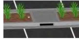
Horizontal Flow Biofiltration System
